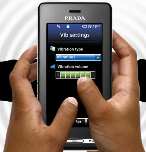
\* Haptics, from the Greek “hapesthai,” meaning “to touch.” Haptics technology used in mobile device user interfaces is also known as haptic, tactile, touch, and vibrotactile feedback.
