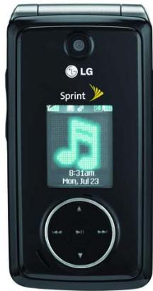
The LG LX570 Muziq uses a capacitive sensing surface for its external music playback controls. The addition of haptic feedback gives users valuable confirmation of their control interactions.
